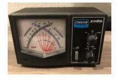
Very Good condition--frequency range: 1.6-200 MHz Input impedance: 50 ohms Power scales: 20, 200 and 2kw. Measures AVG and PEP Power. Includes meter, original box. \$50 (also posted on QRZ—subject to prior sale)
