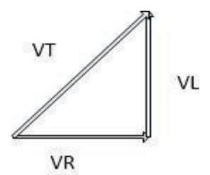
Yeah, yeah, we'll get back to j numbers. In electronics we talk about Real numbers referenced to resistors and Imaginary (j) numbers referenced to inductors or caps. This triangle represents the voltages in the R-L circuit above and we can write a j-number for the circuit.
