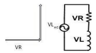
Of course we can't stop there because the question always comes up, what is the total voltage in the circuit. Turns out the total voltage is the hypotenuse of a triangle with the two legs we have, so all together it looks like this:
