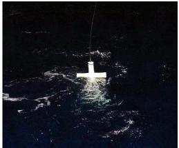
"Over the past year, Randy and I have mentored the MCHSARC in designing and constructing a simple marine buoy that was deployed from the RV *Sally Ride* [on July 16], about 700 kilometers off the coast of southern California," Karn said in a **post** on the AMSAT Bulletin Board. "It is up and transmitting *WSPR* on 20 meters using the call sign KQ6RS, and is being received all over the US and into Canada and Brazil." Karn is **blogging** about the project with updates.
